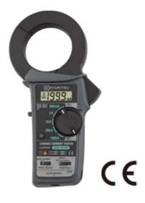
Large transformer jaws of 68mm diameter makes it possible to clamp on all three or four wires (3 phases) together for leakage current measurement.
