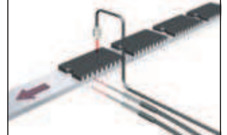
Detection of bends in electronic component leads
